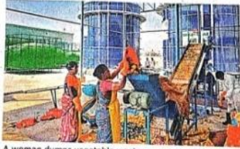
A woman dumps vegetable waste on a conveyor belt that takes them to a biogas plant and a power plant at the Bowenpally vegetable market in Hyderabad. — DC
