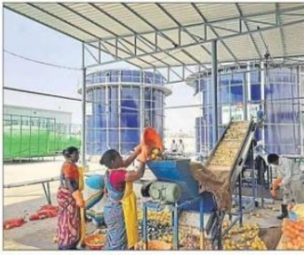
The Bowenpally vegetable market has a power plant that uses vegetable waste to generate power. ■HT PHOTO
