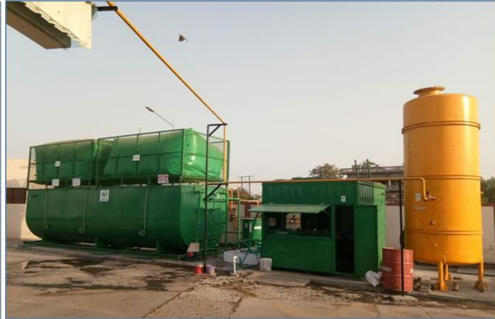
750 kg/day capacity food waste plant at The Akshaya Patra Foundation (Bhavnagar, Gujarat) Generates 40 kg LPG equivalent /day (Installed:2018) Area footprint: 11 m x 3.5 m
