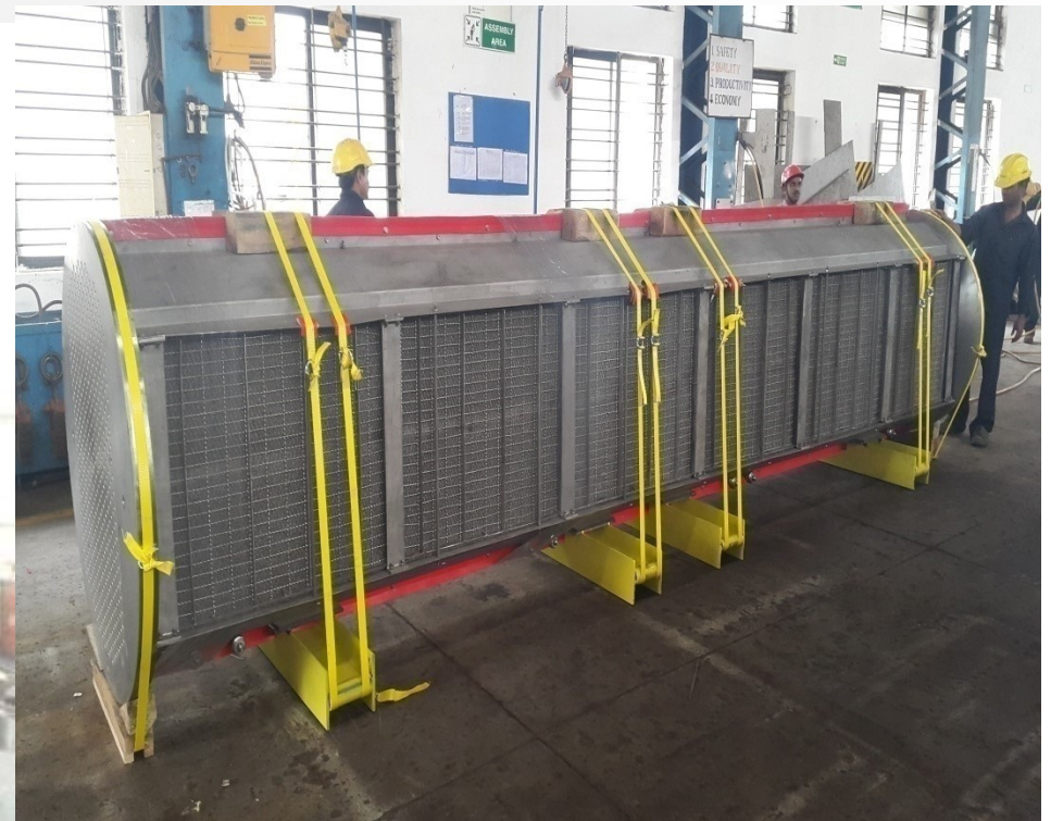
Supply of Tube Bundle to RCF(Mumbai)
